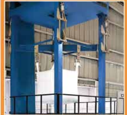
Load Testing machine
